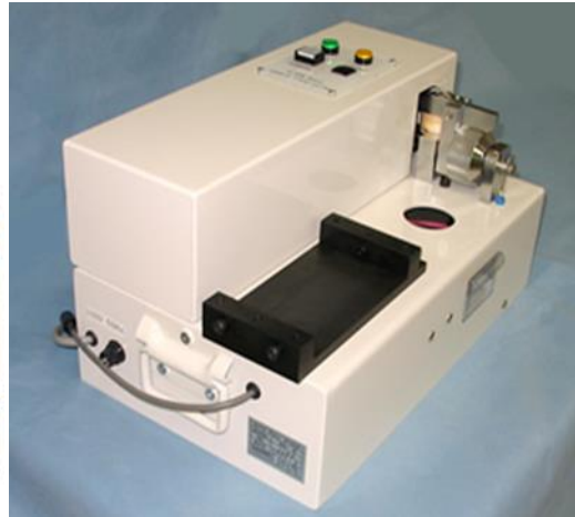
Pull force Gauge TYPE:MS-6
